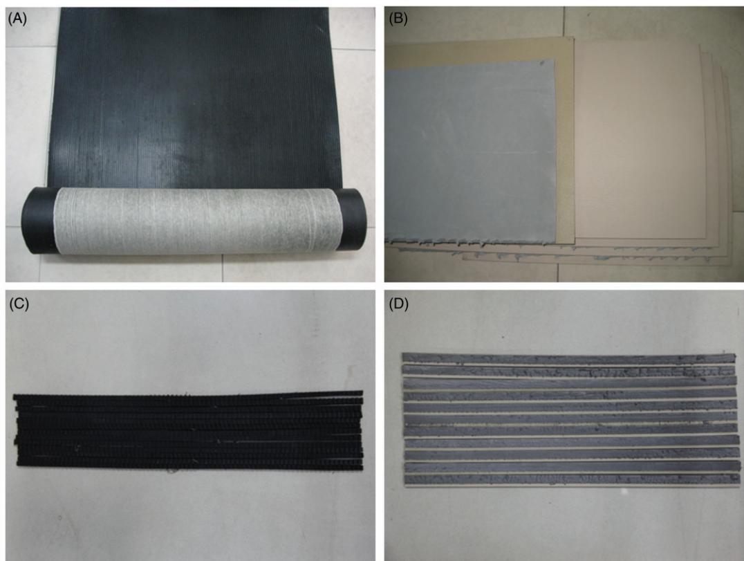
Figure 2. Non-metal materials used in the smoke generation system. (A) Floor glue and its main ingredient is rubber. (B) Heat insulator, including surface layer and inner layer, and the main ingredient is rubber and polyurethane flexible foam, respectively. (C) Floor glue cut into small uniform rectangular pieces with the cross-section of 5 mm × 5 mm. (D) Heat insulator cut into small uniform rectangular pieces with the cross-section of 5 mm × 5 mm.
