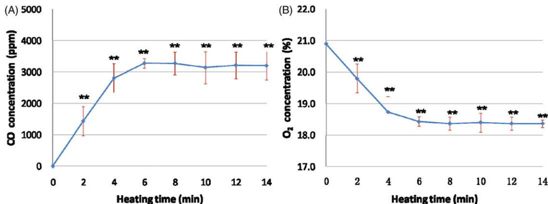
Figure 4. Time course changes of the main inorganic gases in smoke ( $n=3$ ). (A) Changes of CO concentration in smoke with time of combustion. (B) Changes of O<sub>2</sub> concentration in smoke with combustion time. \*\*: Compared with pre-heating time point group,  $p<0.01$ .
